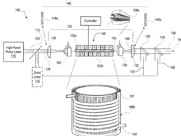
to form a cylindrical fiber assembly. The electrodes are activated to achieve quasi-phase matching.
